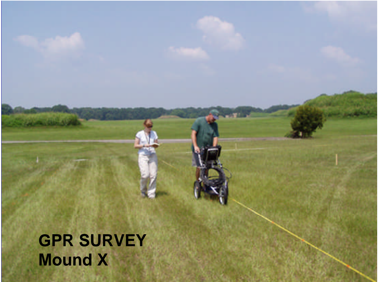
Figure 10. Ground penetrating radar survey.
